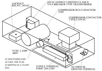
Figure 6: Electric component location.
